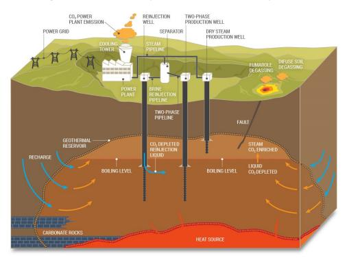
Figure 4: Schematic diagram of a volcanic geothermal system highlighting processes affecting CO<sub>2</sub> emissions as a result of large scale removal of fluid (mass production) from the system.
