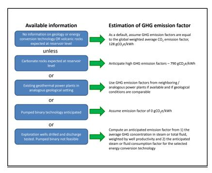
Figure 8: Decision tree for estimating GHG emission factors ex ante for geothermal projects depending on the amount of available information.
