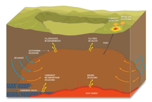
Figure 1: Schematic diagram of a volcanic geothermal system showing the natural sources (recharge, rock dissolution, decarbonization or carbonate rocks or magma degassing) and sinks (dissolution in groundwater, precipitation in calcite, and emission through fumaroles or through soil) of CO<sub>2</sub>.
