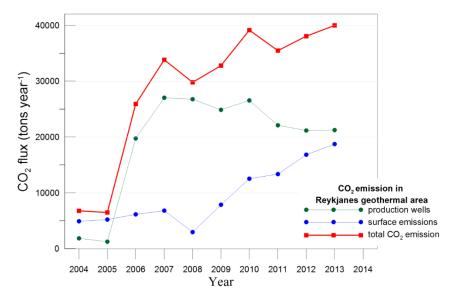
Figure 6: CO<sub>2</sub> emissions from the Reykjanes Geothermal system, Iceland. Red curve show the combined emissions from power production (green) and diffuse CO<sub>2</sub> degassing through surface (modified from Óladóttir and Fridriksson, 2015).
