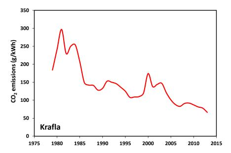
Figure 2: Emission factors from the Krafla geothermal power plant.
