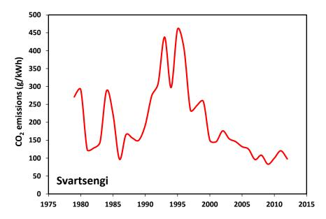
Figure 5: CO<sub>2</sub> emission factors for the Svartsengi geothermal power plant.
